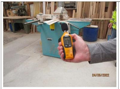
Inside the workshop with the radio and dust extraction switched on, a bandsaw, a circular saw and the planer/thicknesser running. This is equivalent to a full team working. The band is 85 to 90 decibels.
