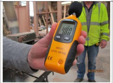
Inside the current workshop at lunchtime ... all equipment, dust extraction and radio switched off. The range is 45 to 50 decibels. This seemingly high band is partly due to proximity to Olivers Transport.
